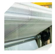
Considering the roll sizes, we can produce the full scope starting from the big jumbo rolls of 500-1500 m in 1-6 m widths to the smallest rewound cut mesh tapes of 0.1 x 10 m roll length.
