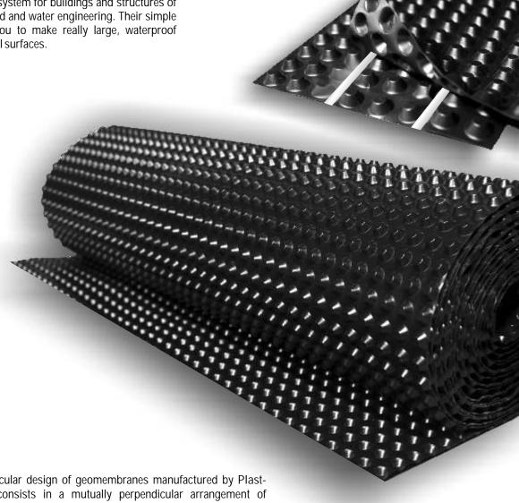
The particular design of geomembranes manufactured by Plast-Master consists in a mutually perpendicular arrangement of dimples, called an orthogonal system. It provides maximizing the water flow in the plane of the product, facilitates installation within the area of plane bends, increases the tensile strength, especially within the fabrication direction, compared to the diagonal system. It gives the opportunity to make a so-called, modular seam.
