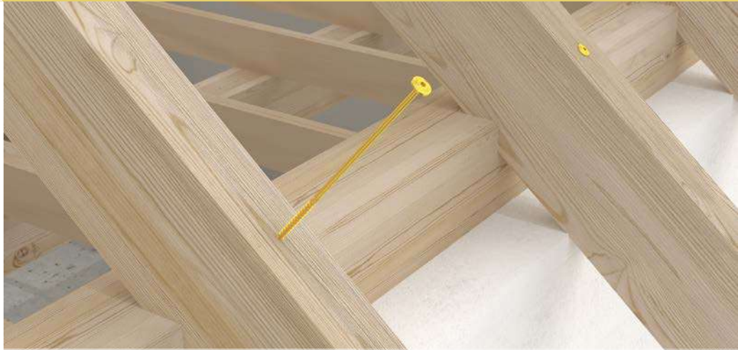
▶ CONNECTING RAFTERS WITH PURLINS
