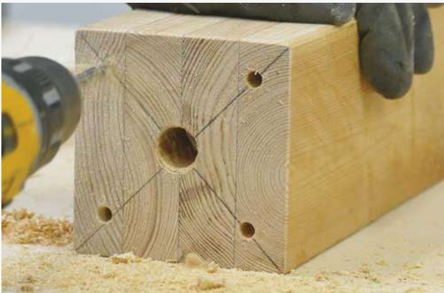
4 Reaming holes for wood screws.
