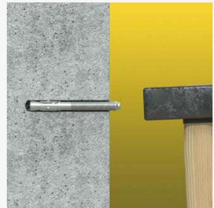
3 Place the anchor in the drilled hole.
