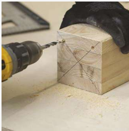
2 Reaming holes for wood screws.
