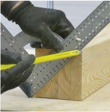
1 Determination of post diagonals.
